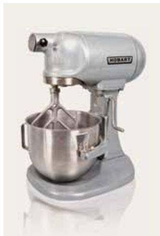
**Mortar test:** to evaluate the air content of emulsions for mortar application used
