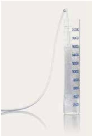
**Sintered glass test:** to select appropriate antifoams for water-based polymerisation
