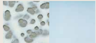
Wetting of siliconized substrate without additive with TEGOPREN® 5840
